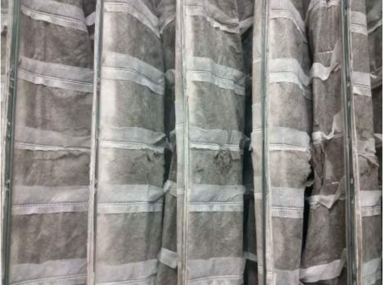
Image 2: UVDI Charcoal Bag Filter with holes burned by UVDI Lamp.
