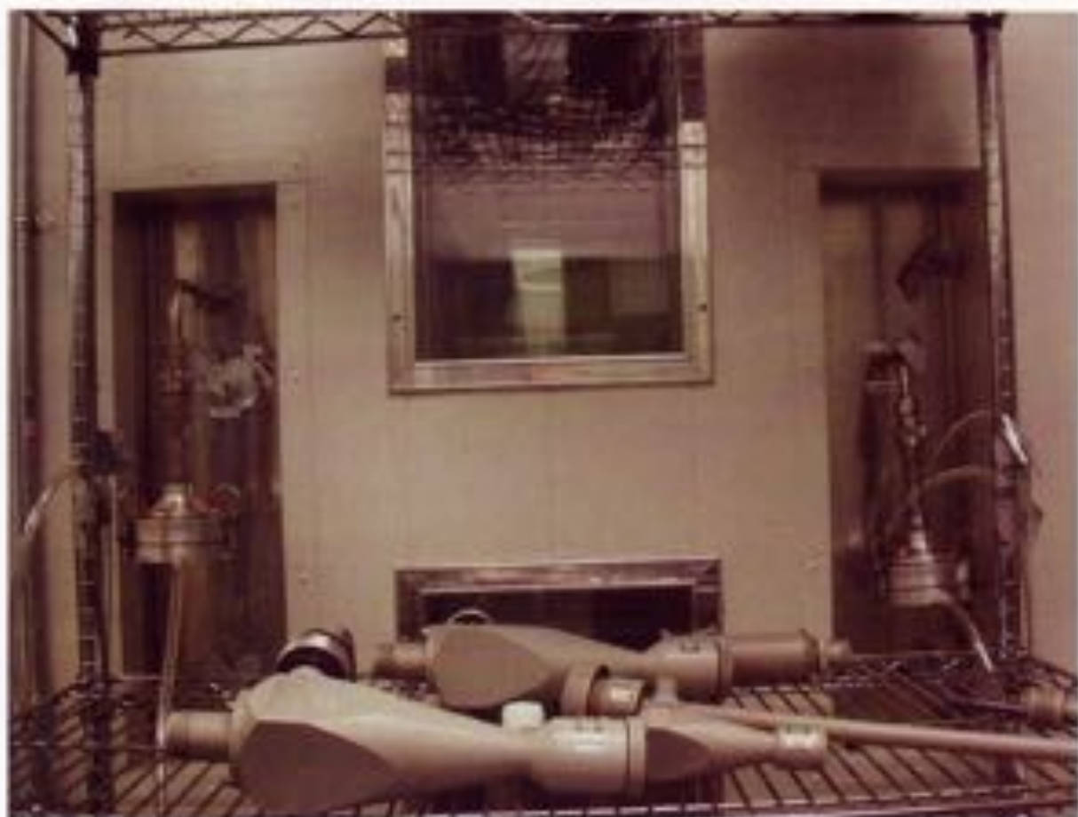
Photograph 2. View of Samplers in Test Positions at Chamber Wall. Each of two Anderson single-stage impactors used for S_e and A_v sampling is visible at the sides of the photo. Air samples are extracted from the chamber through tubes that lead to the samplers through ports in the chamber wall. The flexible tubing connected to the bottom of each sampler leads to vacuum pumps that regulate the flow of extracted air.
