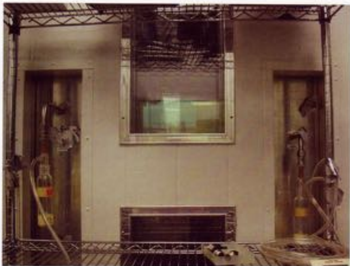
Photograph 3. View of Samplers in Test Positions at Chamber Wall. Each of two all glass impingers used for MS2 sampling is visible at the sides of the photo. Air samples are extracted from the chamber through tubes that lead to the samplers through ports in the chamber wall. The flexible tubing connected to the bottom of each sampler leads to vacuum pumps that regulate the flow of extracted air.
