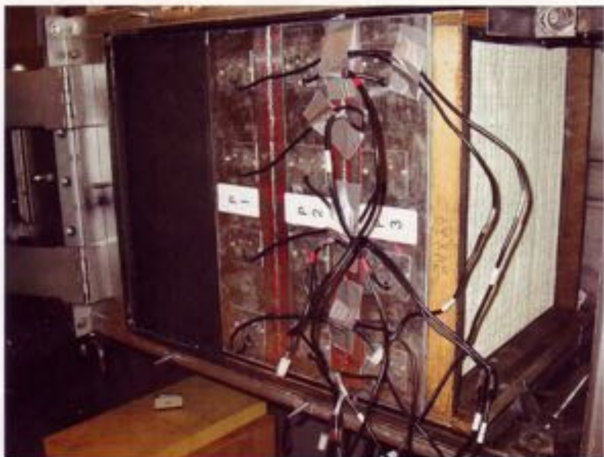
Photograph 4. View of sequential photo-catalytic oxidation sections installed in test duct. Air flow in the test duct is from left to right. The black section directly upstream of the device is the light baffle. Adjustable mechanical clamps and wooden force-transfer elements visible at the right of the photo secure the test assembly against a gasketed flange within the test duct. The entire side of the test duct section shown is covered by a sealed panel, through which the electrical cords pass.
